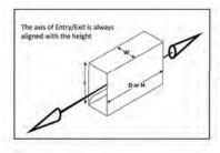
All folding cartons have at least one panel covering the end or ends, usually with a flap that tucks into the piece to keep the lid closed. The point where this top panel pivots is always the length dimension. In the case of a sleeve, the height is always aligned with the axis of the open end or ends. This also applies to cartons and other packaging like
