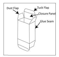
Tuck- These are the narrow panels that are attached to the top and/or bottom covers that tuck into the body to keep the covers closed. Usually rounded or tapered on the covers
