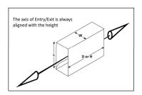
All folding cartons have at least one panel covering the end or ends, usually with a flap that tucks into the piece to keep the lid closed. The point where this top panel pivots is always the length dimension. In the case of a sleeve, the height is always aligned with the axis of the open end or ends. This also applies to cartons and other packaging like trays too.
