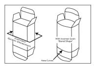
Most often the grain direction of a folding carton is aligned perpendicular to the glue seam. If grain alignment is incorrect, the carton can get "barrel shaped".
